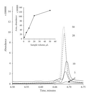
FIGURE 1: Effect of introduced sample volume on the resulting fullscan caffeine GC/MS response. Numbers represent sample volume in  $\mu$ L. Insert plot of peak area vs. sample volume.
