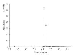
FIGURE 2: Typical chromatogram obtained for a  $5 \,\mu$ L sample of  $117 \,\mu$ g/mL caffeine (i) with lidocaine, internal standard (ii).
