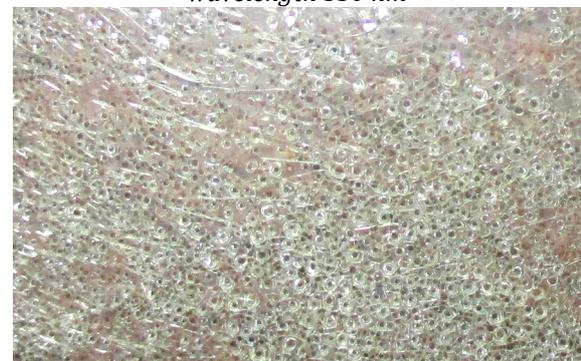
*After the impact of laser radiation with the wavelength 650 nm*
