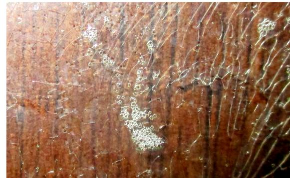
*After the impact of laser radiation with the wavelength 530 nm*
